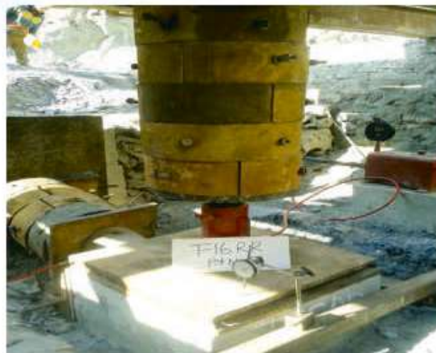
Rock to Rock Block Shear Test at Dam Site of Vyasi Hydro Electric Project (Uttarakhand)
