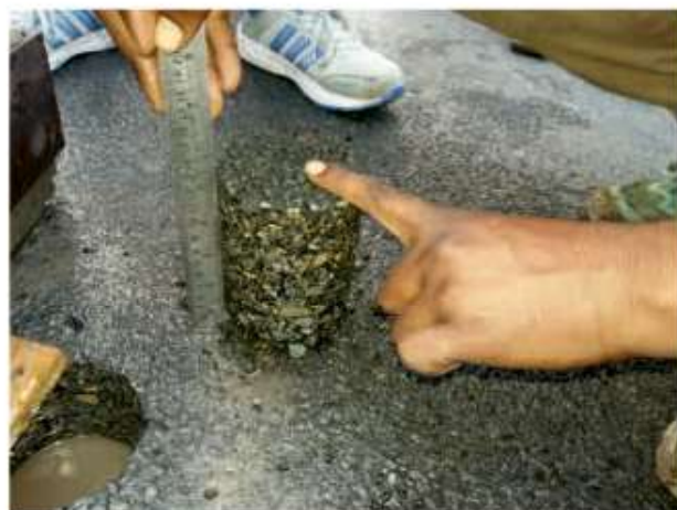
Core Cutting of Bituminous Pavement
